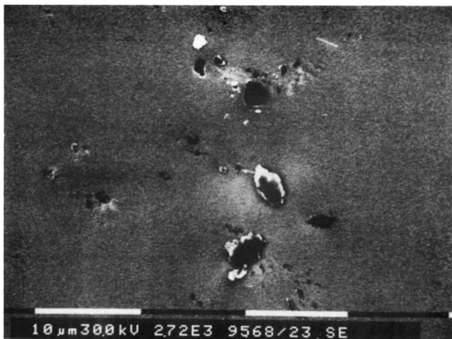
Fig. 9. A scanning electron microscope (SEM) picture of a plasma polymerized acrylic acid layer (5 W) after separation from molecular contact during adhesion force measurement; the picture shows tiny lumps and pits indicating material transfer during separation.
